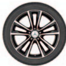
5-twin-spoke light-alloy wheel, painted black and with a high-sheen finish, with 225/40 R 18 tyres (optional, integral part of Night package), Code 01R
